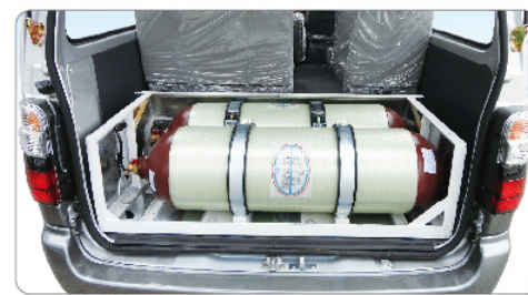
2×80L Gas Cylinders
